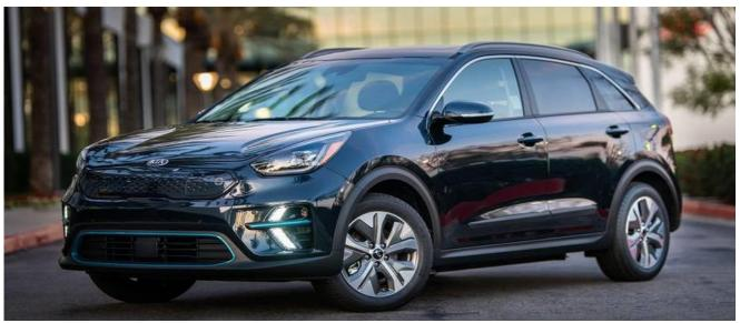
The 2020 Kia Niro EV is a fully electric version of, yes, Kia's Niro. Kia also sells the Niro as a regular hybrid as well as a plug-in hybrid, but the EV only uses electricity. For power, it uses a 64-kWh battery with a 201-horsepower electric motor that drives the front wheels.
